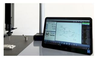
The Touch Screen user interface makes measurements easy and straightforward.
